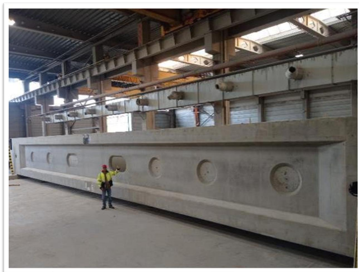
Prefabricated columns, Baltic Towers, Mszczonów production plant
