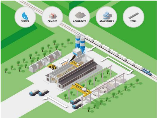
A scheme of manufacturing of the prefabricated reinforced elements by Pekabex BET S.A
