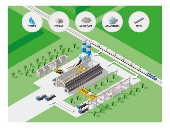
A scheme of manufacturing of the prefabricated structures: single-, doubleand triple-layered walls by Pekabex BET S.A.
