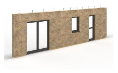
Triple-layered walls with texture consist of carrying, insulating, and facade layers. Additionally the facade layer is finished with mineral plasters, washed stone, or imprints of decorative stencils. The prefabricated elements may have holes for windows and doors practically in any dimensions and shapes. Depending on the element thickness and method of filling the joints the fire resistance is up to REI 240. Walls are available in various sizes and different types of insulation.
