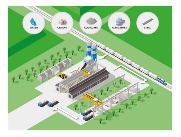
A scheme of manufacturing of the prefabricated filigree slabs by Pekabex BET S.A.
